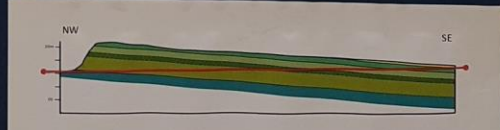
Figure 2: Schematic geological cross section through the Chilterns. Different chalk formations dip gently to the south, forming the northern rim of the London Basin. The red line shows how any proposed rail route would tunnel/cut from younger to older chalk passing from the southeast to the northwest.
