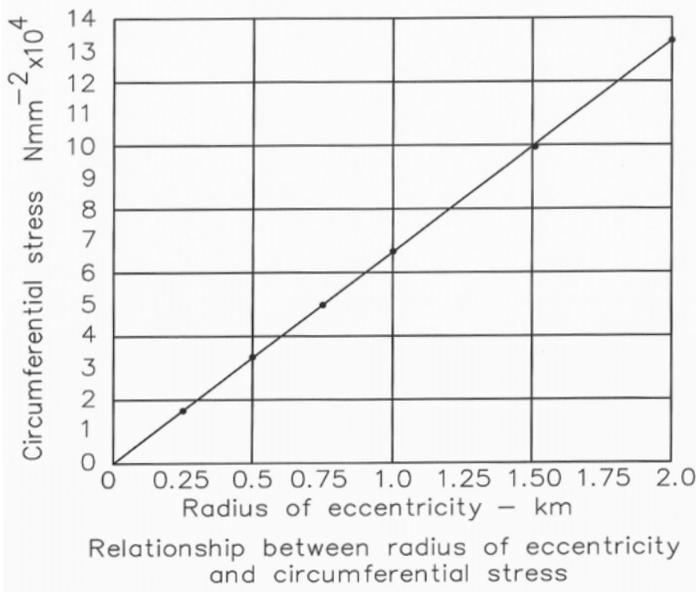
**Fig 36: Relationship between the radius of eccentricity & the circumferential stresses**
