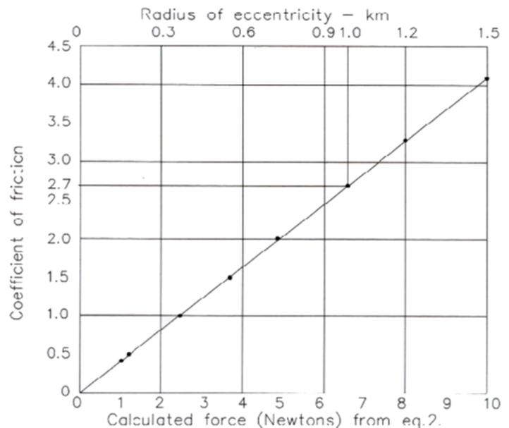
**Fig 37: Relationship between the force (Newtons) needed to move a 1km x 1m x 1m element of crust and the coefficient of friction at the crust/mantle interface**
