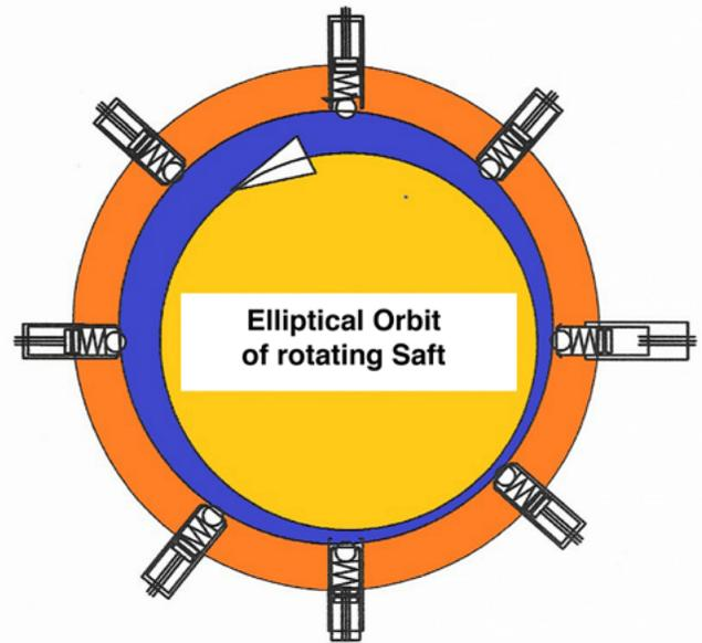
Displacement & Vibration detectors around shaft & bearing supports
