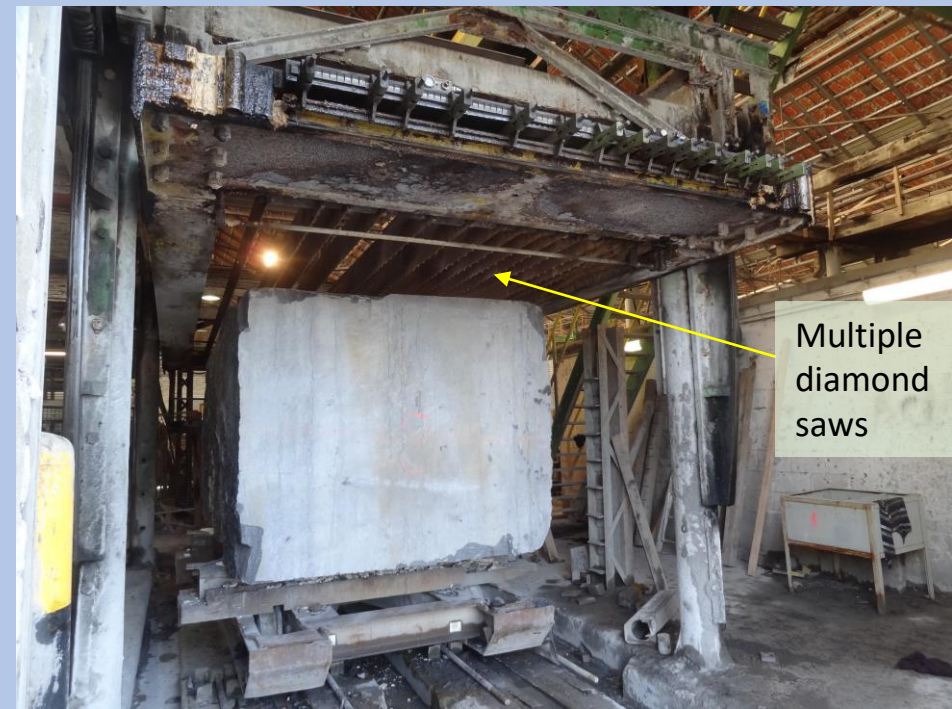
Upper L: Blocks to be sawn into slabs. Lower L: Block in place for sawing. Above: Sawing completed (takes about 1.5 hours) The water-cooled* saws move back and forth; their spacing can be adjusted for the slab thickness required. This machine, one of several, has 68 saw blades.
