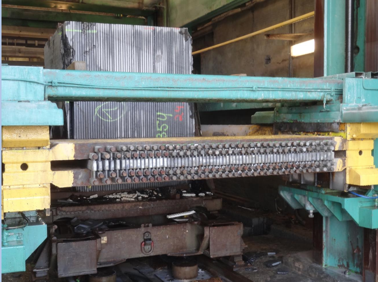
Upper L: Blocks to be sawn into slabs. Lower L: Block in place for sawing. Above: Sawing completed (takes about 1.5 hours) The water-cooled* saws move back and forth; their spacing can be adjusted for the slab thickness required. This machine, one of several, has 68 saw blades.
