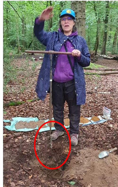
Screw auger was used for the final sample from 76cms
