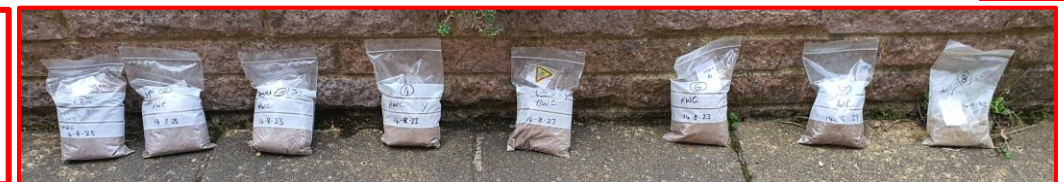
Bagged samples to be sent for analysis. The rest was returned to backfill the hole.
