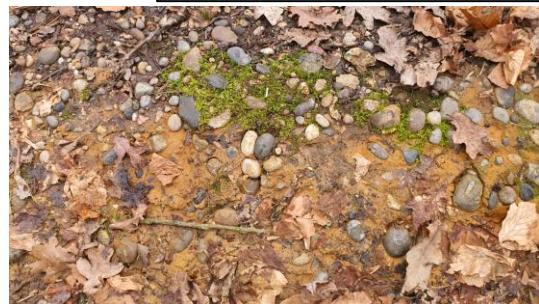
Top of ridge: Gravel has clayey matrix
