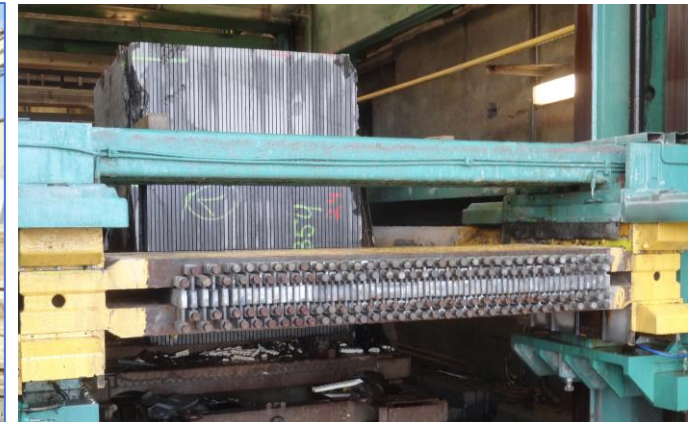
Hainaut Quarry, Belgium. Stone block being sawn into multiple slabs and stone slabs awaiting further processing.
